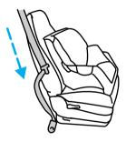
3. While holding the shoulder and lap belt portions together, route the tongue through the child seat according to the child seat manufacturer's instructions. Be sure the belt webbing is not twisted.
